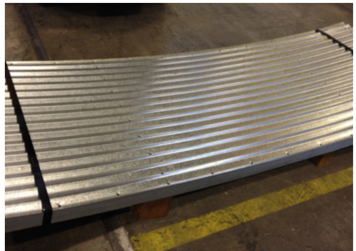
Figure 3: New silo wall sheets ready for shipment
