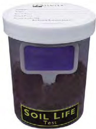
The paddle inside Solvita's soil-testing jar changes color to indicate CO 2 levels.
