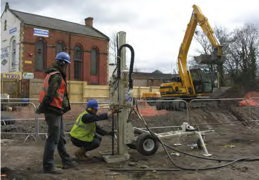
Fig 9 Undertaking the geoarchaeological survey with the Geoprobe drilling rig
