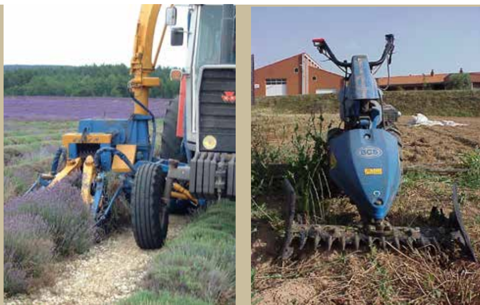
Figures 37, 38. Specific harvester for Lavandula sp. (left) and cutterbar added to a motorized plough (right).
