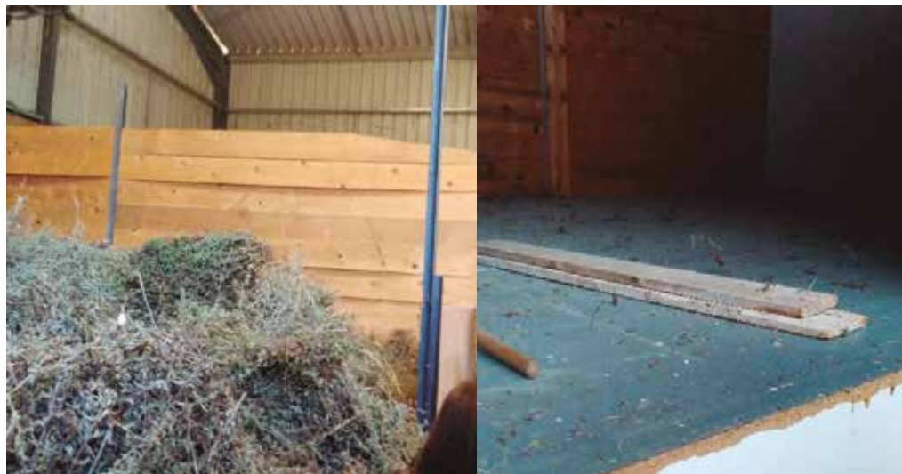
Figurex.7. Drawer dryer (hot air passes below the plant pile).
