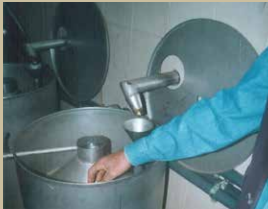
Figures 55, 56. Steam distillator boiling chamber and discharging system.
