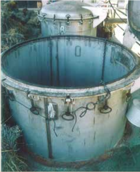
Figures 55, 56. Steam distillator boiling chamber and discharging system.
