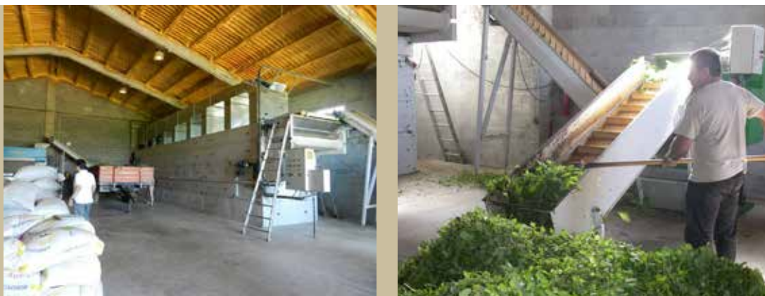
Figures 47, 48. Continuous dryer by conveyor system
