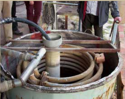
Figures 57, 58. Cooler and essential oil separator elements.
