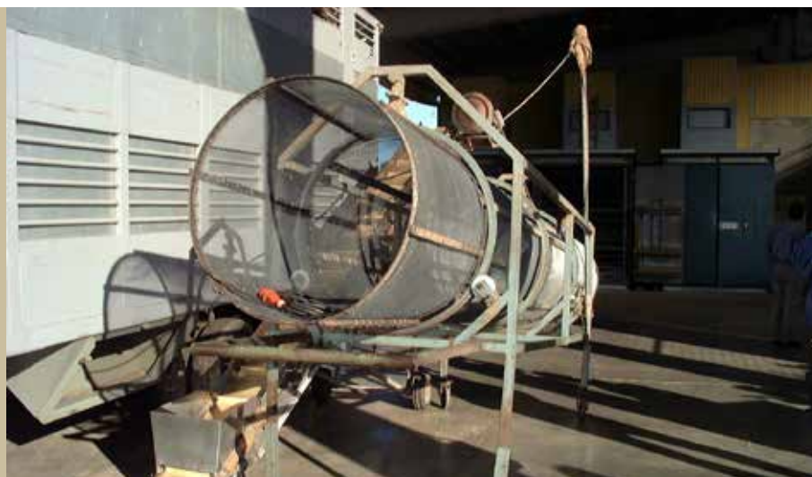
Figure 41. Cylinder with different sieve opening for remove soil from herbs.
