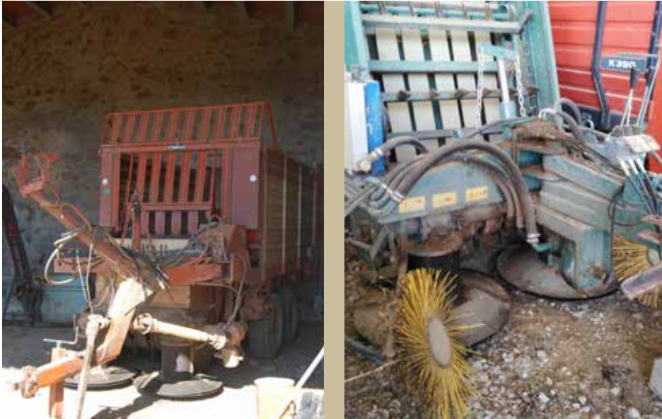
Figures 39, 40. Forage harvester used for MAPs (left) and brushes adapted to a forage harvester (right) to lift the plant sides.
