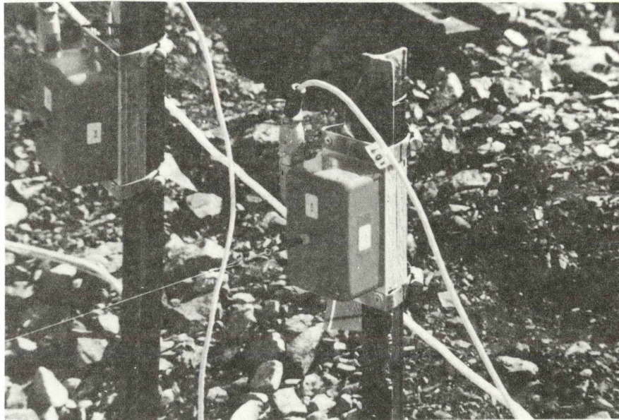
Fig. 15 - DISPLACEMENT TRANSDUCERS, INSTALLED
