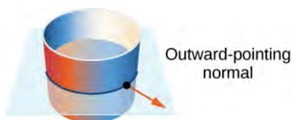
Figure 6.75 If all the vectors normal to a cylinder point outward, then this is an outward orientation of the cylinder.
