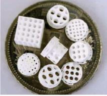
Figure 1 Diverse calcium phosphate-based bone substitutes produced by additive manufacturing (Ghayor & Weber FE (2018); Frontiers in Physiology doi: 10.3389/fphys.2018.00960)
