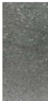
Figure 3 Dull Gray Passivated Zinc
