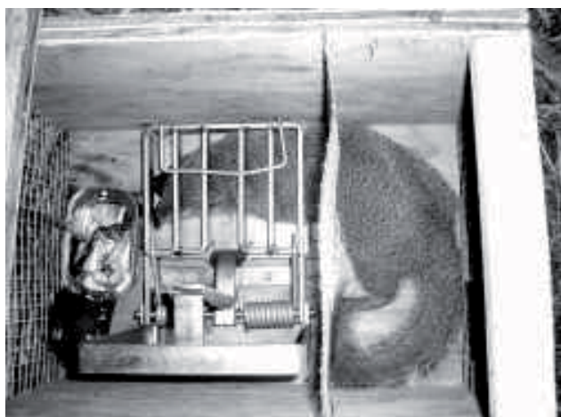
Fig. 2 DOC 250 kill trap baited with sardines. The small Indian mongoose has been humanely killed.
