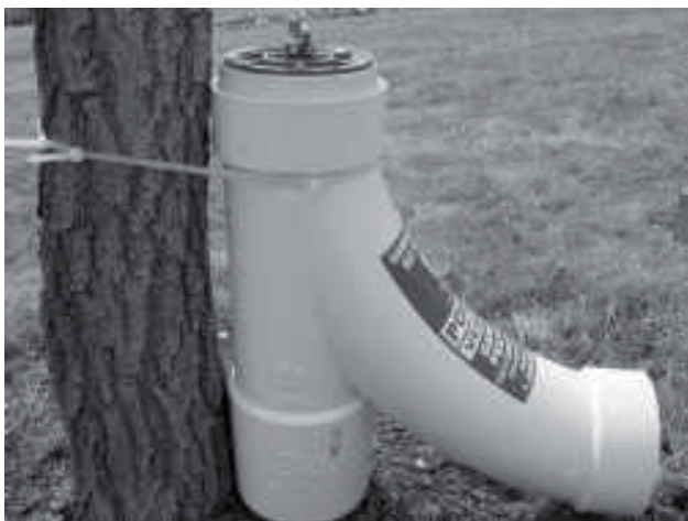
Fig. 2 Bait station designed and used in the Gambian giant pouched rat eradication attempt on Grassy Key, Florida.
