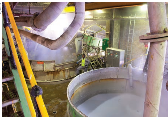
A repulper contains the waste paper, water, de-inking agents and chemicals and softens paper fibres into a slurry.
