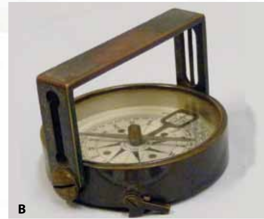
Figure 2.1. U.S. Geological Survey (USGS). Top row: (A) detail from a Meganos land grant map by A.W. Von Schmidt in 1861; (B) a surveying compass which was used by early surveyors to measure direction; and (C) a portion of a USGS map near Antioch. (D) Surveyors in the field ca. 1925 working with an alidade and a plane table. The alidade was used to sight an object and draw a line or angle on the plane table during the construction of a topographic map. (A: Los Meganos land grant map, courtesy The Bancroft Library, UC Berkeley; B: courtesy U.S. Geological Survey; C: USGS 1918 (Collinsville), D: USGS ca. 1925, courtesy U.S. Geological Survey)
