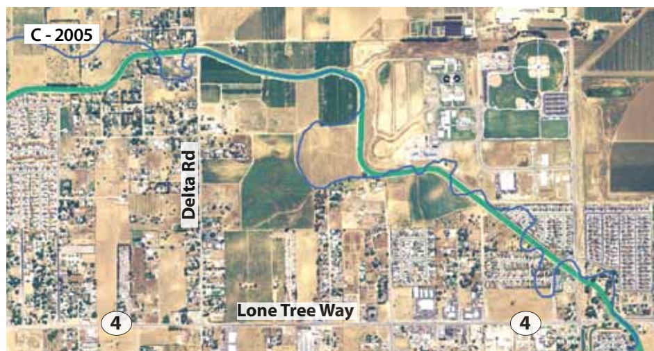
Figure 4.11. Modifications to Marsh Creek. The engineering map (A) shows a 1959 design to remove several meanders from Marsh Creek. These meanders can clearly be seen in the historical aerials (B) and have been removed today (C). In B and C the historical network is shown in blue, overlaid on the present day network shown in turquoise. D) A crew of men installing pipe in Contra Costa Canyon demonstrate another type of human impact on streams. (A: Eastern Contra Costa Soil Conservation District et al. 1959; B: USDA 1939, courtesy of Contra Costa County and the Earth Sciences & Map Library, UC Berkeley; C: USDA 2005, courtesy of NAIP; D: Sanderson & Porter 1915, courtesy of Contra Costa County Historical Society)
