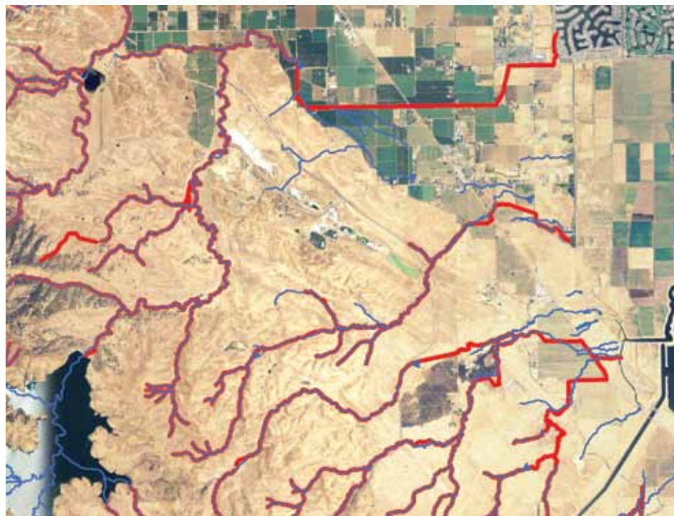
Figure 4.10. Changes in the southeastern drainage network. The contemporary network (shown in red) of Kellogg and Brushy creek watersheds has extended and straightened portions of the historical network (blue) to make it much more continuous. (USDA 1939, courtesy of NAIP)
