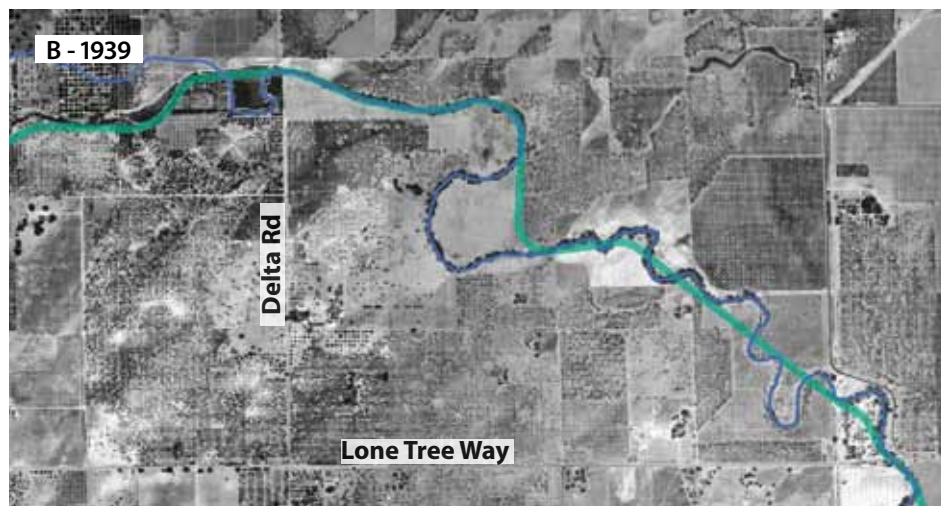
Figure 4.10. Changes in the southeastern drainage network. The contemporary network (shown in red) of Kellogg and Brushy creek watersheds has extended and straightened portions of the historical network (blue) to make it much more continuous. (USDA 1939, courtesy of NAIP)
