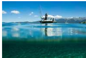
Without a propeller and with its shallow draft, DRI's jet boat nearshore research vessel allows scientists to study changes in water clarity and other important nearshore characteristics in the shallow areas of the lake.
